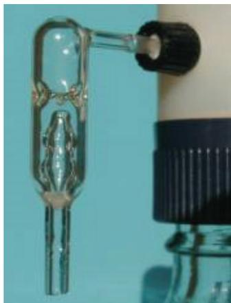
Borosilicate glass one-way valve with plastic coating, avoids the emission of gases and strong smells
